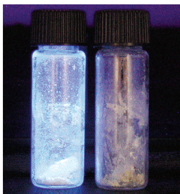
FIGURE 7. Xerogels 2 obtained upon bubbling CO 2 to benzene (left) and benzene–nitrobenzene 95:5 (right) solutions of 1 .
